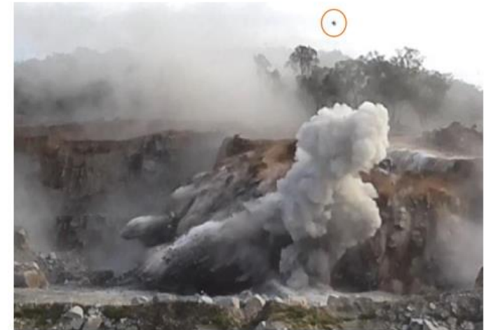
Figure 9 - Flyrock landing in dam in front of firing location
