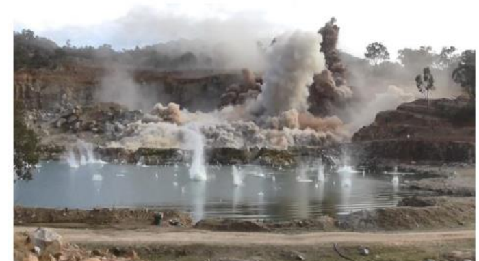
Figure 9 - Flyrock landing in dam in front of firing location
