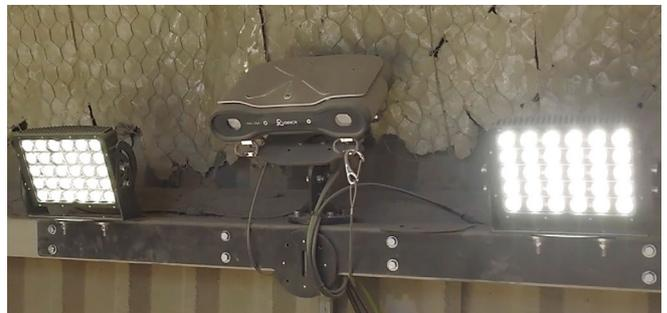
Figure 2 - FRAGTrack™ Lightweight F60 Camera and F50 Processing Unit mounted at Drury
