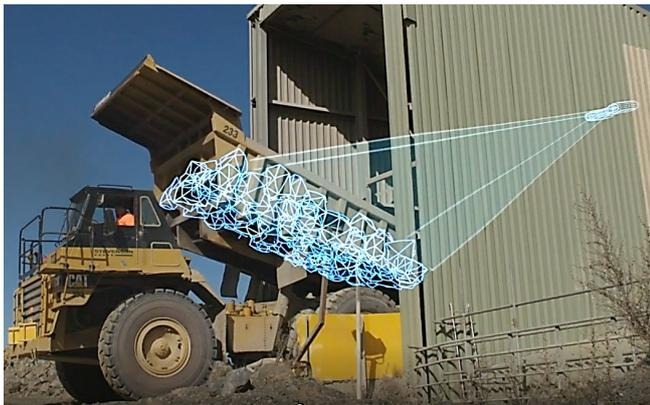
Figure 3 - FRAGTrack™ captures a sample during tipping operation.
