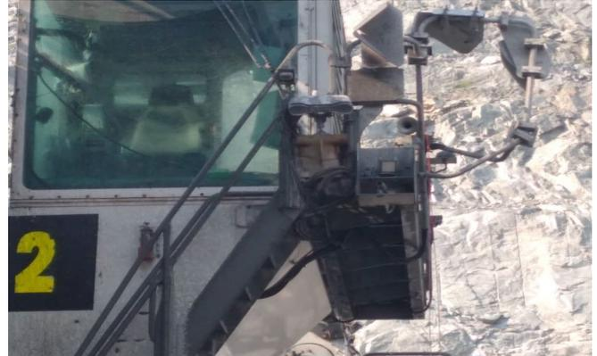
Figure 3: F60 camera unit mounted on EX002
