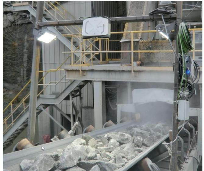
FRAGTrack™ installed next to the primary crusher
