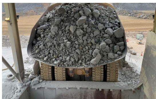
FRAGTrack™ Crusher camera view. Measurements are captured and processed in real-time during the tipping operation.
