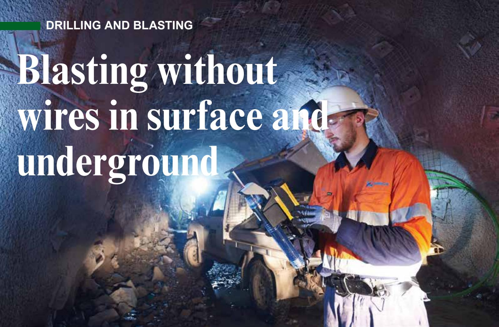
A WebGen™ unit is encoded at CMO Northparkes mine by an Orica engineer, ready for loading.
