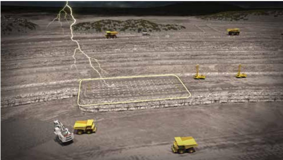
Wireless blasting with WebGen™ significantly reduces the risk of lightning initiation in a blast hole.
