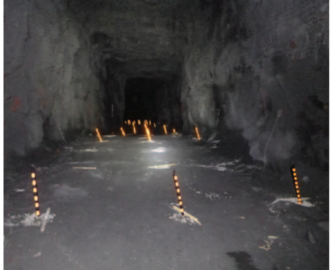
Left: a drift at Goldcorp's Musselwhite mine loaded for blasting using traditional methods. Right: a drift at Musselwhite loaded for blasting with Orica's WebGen wireless system.
