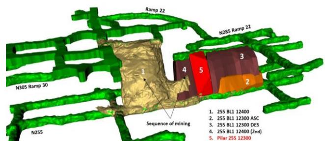
255 BL1 12300 *island [rib] pillar* recovery using wired detonators would be dependent on rock filling the adjacent open stope, reinstalling ground control where needed, scaling, and managing the risks associated with personnel exposure to previously blasted rock mass. This incurs additional costs and time delays. All these operations aim to allow the safe re-entry to the upper level to load 110mm downholes, program the electronic detonators and fire the shot.
