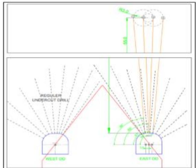
Figure 2. Conditioning blast design (Orange Lines with dotted lines being undercut) at DMLZ.
