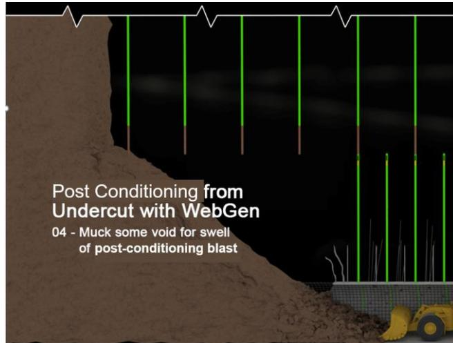
Figure 3. Post Undercut Conditioning Concept
