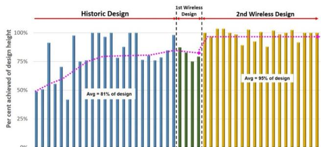
Figure 2 Step change performance following continuous improvement application of WebGen™ in rise/slot widening blasts
