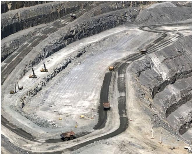
Figure 1 - Production constraints limit areas for blasthole drilling.
