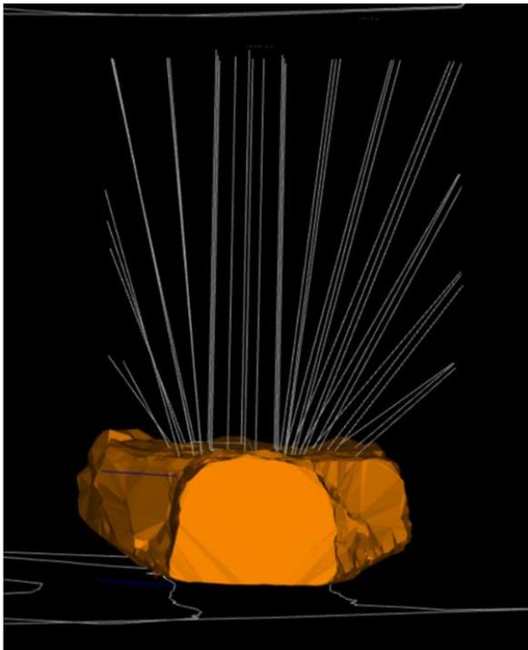
Figure 5. Transverse stope. Widenings blasted and loaded.
