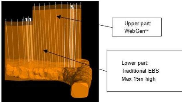
Figure 1. Drill design and block model for 27m high longitudinal double layer blind up hole stope.
