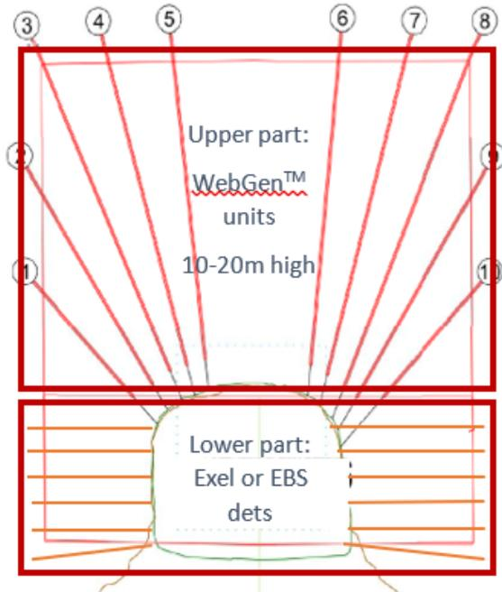
Figure 4. Drill design for transverse Double layer blind up hole stope.
