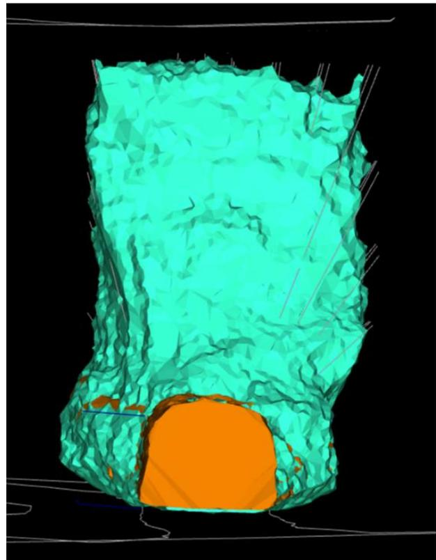
Figure 6. Transverse stope. Blast results after the second (upper) part.
