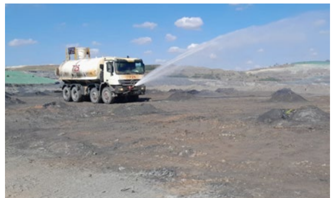
Figure 5 – Truck spraying water on the loaded blast pattern.
