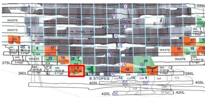
Figure 1: Borden mine layout of the Western Zone (WEZ), looking North
