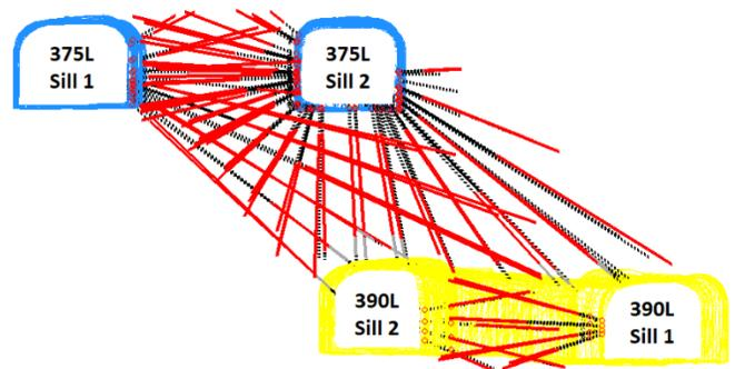
Figure 2: Complex drill design involving all sills
