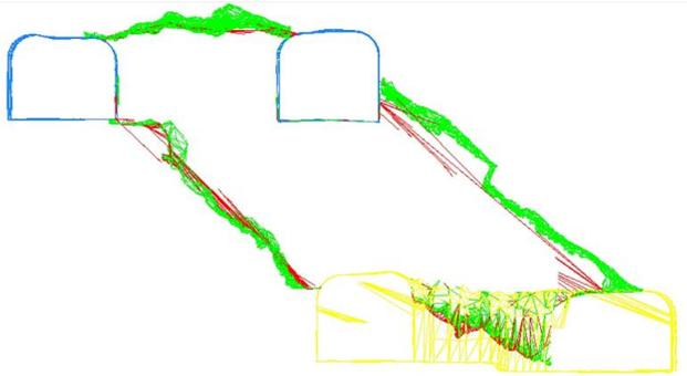
Figure 4: 98% post-blast CMS (Green) vs. designed blast shape (Red)
