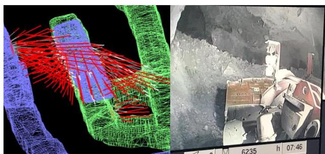
Figure 3: Stope design and mucking horizon post blast
