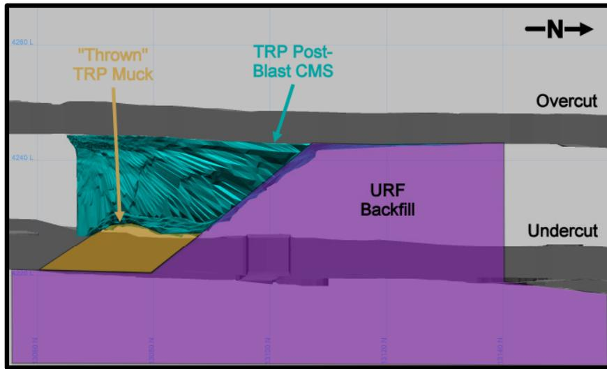
**Figure 9. Longsection view of post-WebGen™ blast CMS**
