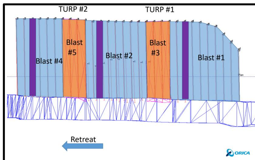
Figure 10. Longsection view of Temporary Uphole Rib Pillar (TURP) mining concept
