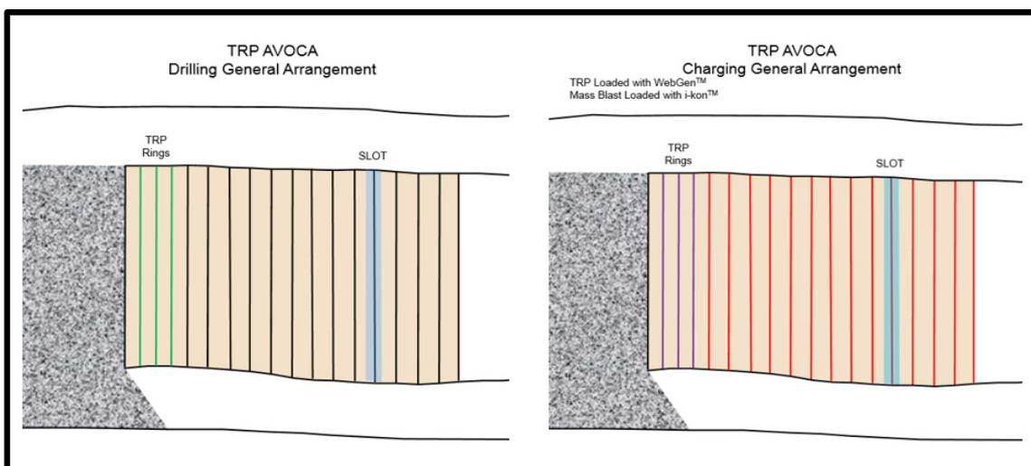
**Figure 2. Schematic of typical drilling and charging arrangement of TRP AVOCA**
