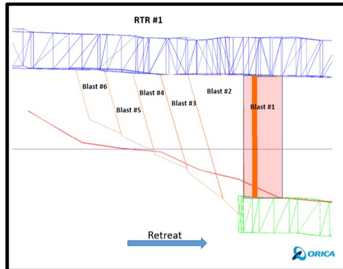
**Figure 11. Longsection view of Reverse Throw Retreat (RTR) mining concept**
