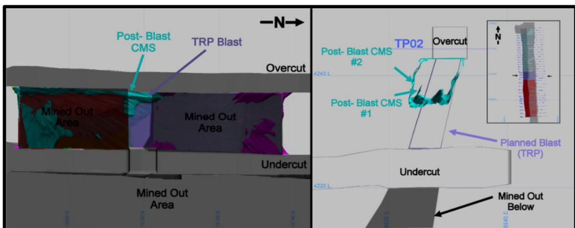
**Figure 8. Longsection (left) and cross section (right) views of TRP WebGen™ blast CMS**
