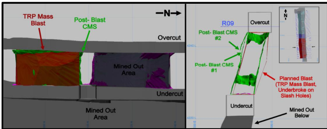
**Figure 7- Longsection (left) and cross section (right) views of TRP stope mass blast CMS's**
