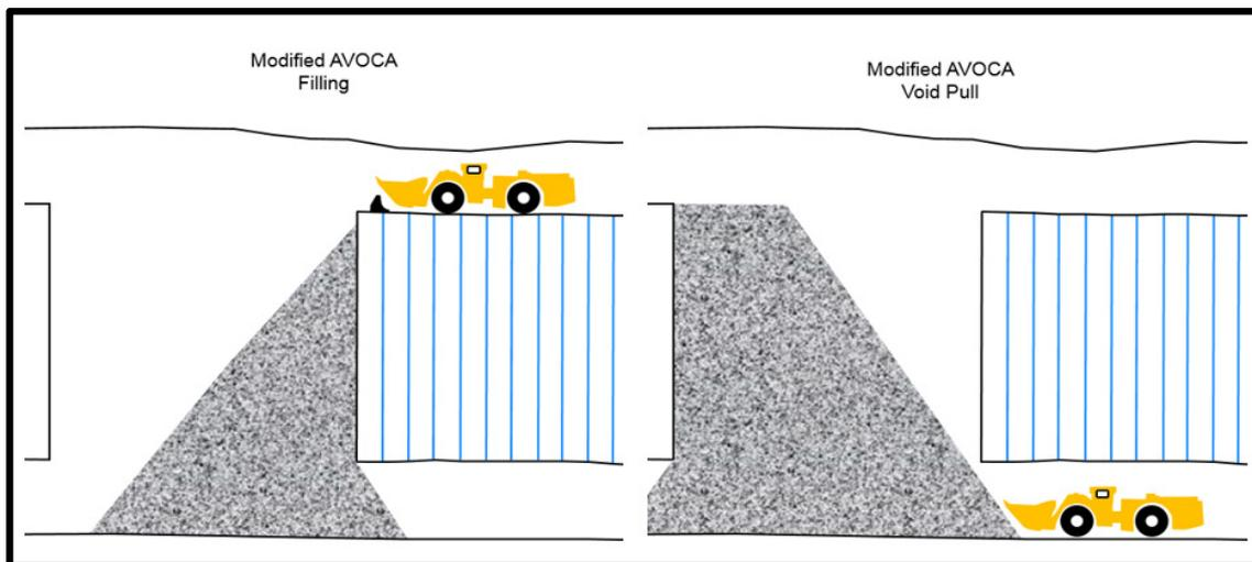
**Figure 1. Schematic of Modified AVOCA filling and void pull activities**
