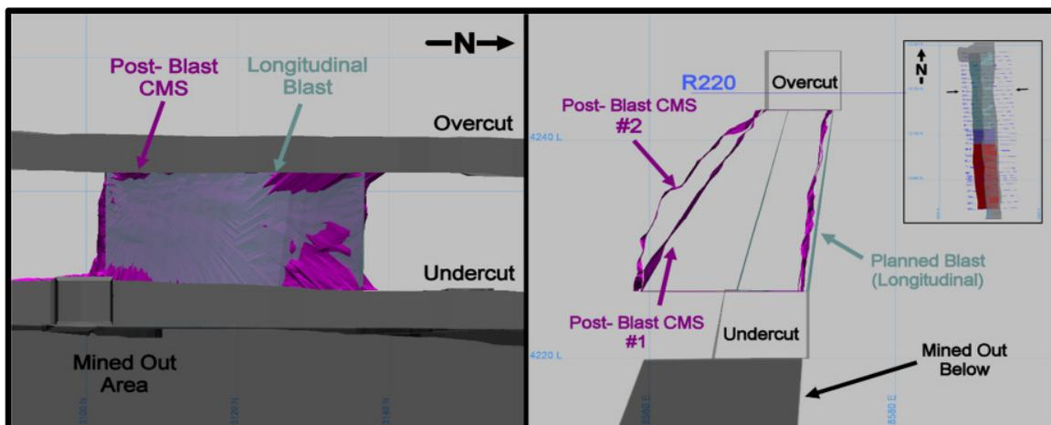
Figure 6. Longsection (left) and cross section (right) views of longitudinal stope blast CMS
