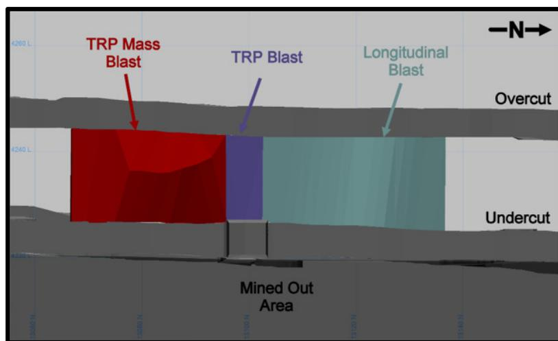
Figure 5. Longsection view of case study stope
