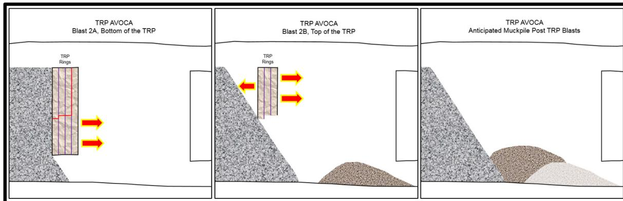
**Figure 4. Schematic illustrating firing sequence of the TRP rings**
