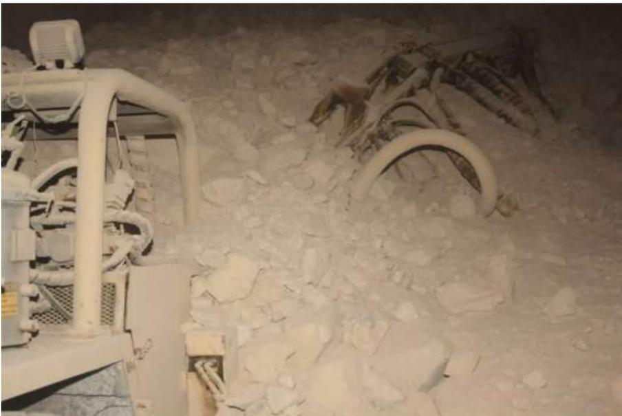
Figure 4. Charge vehicle at SLC mine after an inflow
