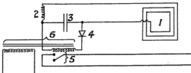
Figure 1. An image illustrating the wireless receiver from an early patent for a directly initiated detonator.
