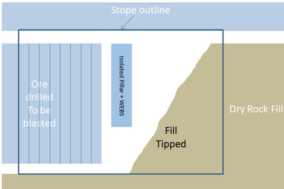
Figure 8. Long Section of Modified Avoca Stope with isolated pillar charged with wireless for later extraction
