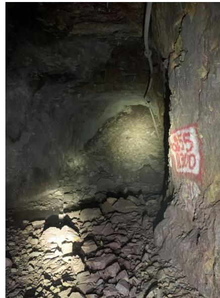
The preloaded pillar had dimensions of approximately 25x30x6m, generating 18.8 kton of ore accounting for 12% of zinc production for the month, achieving an overall average Zn content of 9,19%. Applying WebGen™ 100 enhanced pillar recovery enabled the mine to improve its productivity without exposing people to areas previously damaged due to prior blast cycles.
