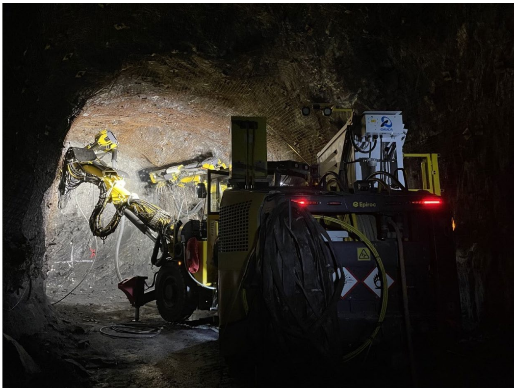
Avatel™ at the face charging
