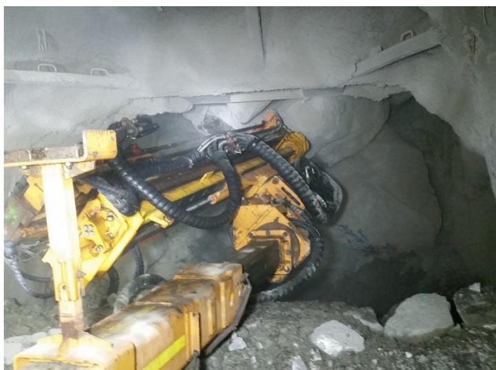
*The Auto Explosive Loader drilling a rock and pushing wireless explosives into the hole.*
