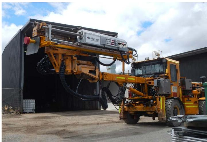
*Cadia's Secondary Break trial using MacLean's Auto Explosive Loader enabled with Orica's WebGen™ wireless technology.*
