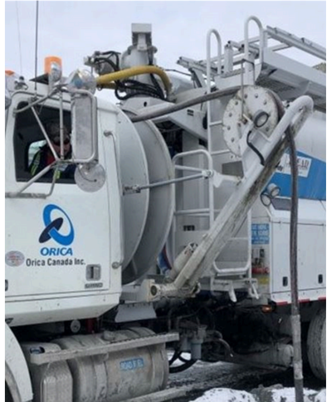
Figure 4 - Fortis™ Protect delivers a special emulsion blend from a modified MMU™.
