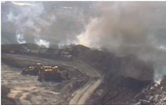
The Liddell Seam is susceptible to spontaneous combustion and although the mines were sealed on cessation of operations, combustion still prevailed. This combustion is fuelled by added oxygen caused by current mining operations. The old workings in the Liddell seam are now being mined to recover the remnant coal left behind in pillars and to allow access to the lower Barrett seam. Failure to remove these areas results in significant loss of reserves and therefore revenue to the owner.
