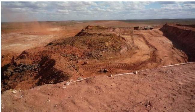
As the Mary Mac pit deepened, Orica were requested to assist with design, loading and firing the second Crown Pillar at the 485 RL. Due to mine planning, this shot was a much more conventional design incorporating a Vertical Crater Retreat slot that fired into the void below with the surround holes firing towards the free face created.
