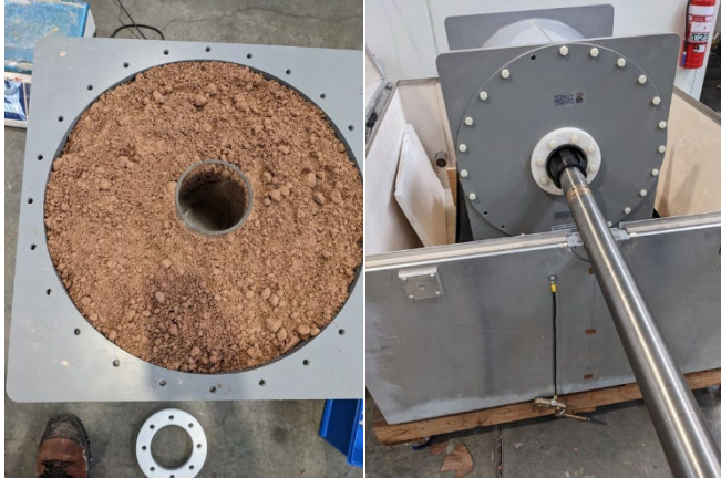
Lab Test Setup: Test vessel during filling (Left) and during WIREBmr™ tool insertion (Right)
