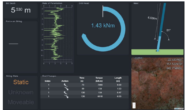
DRILLHub™ live user interface helps users to better plan field operations in real-time.
