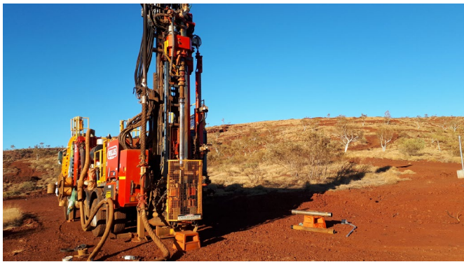
Figure 1. DRILLMax™ alongside the rig – real-time downhole geophysical and directional data while drilling
