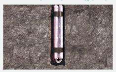
**5.1** Alternate option uses an electronic detonator in toe charge.
