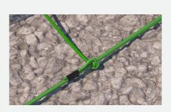
2.2 Tie downline to trunkline. When using only one trunkline, initiate from both ends.
