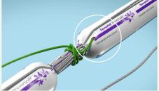
**1.6** Tie detonating cord below first cartridge. Insert tail of detonating cord into the cartridge.
