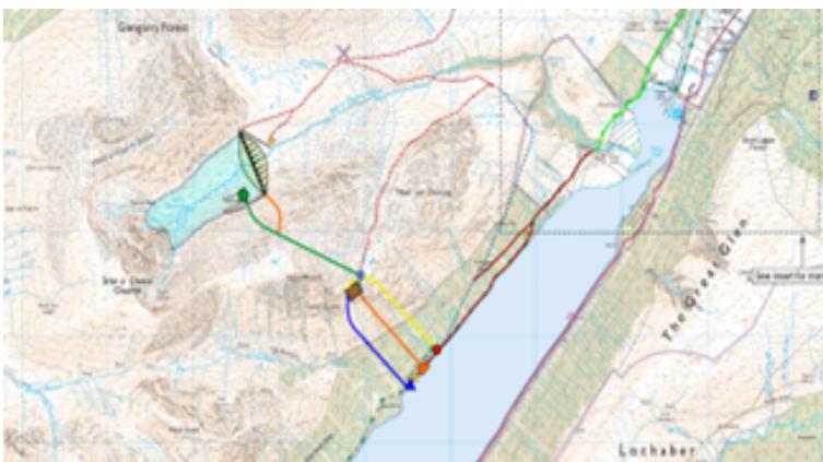
Image 1: Coire Glas Pumped Storage Scheme: over 500m vertical height difference between the proposed upper reservoir and lower reservoir Loch Lochy.
