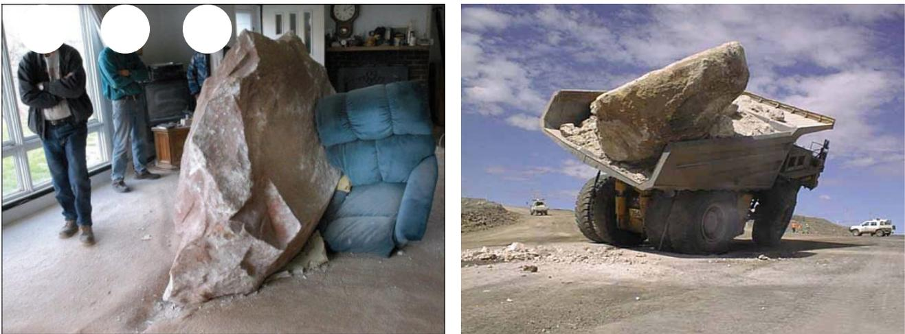
Figure 4: Extreme examples of the hazards of flyrock and of oversized fragments
