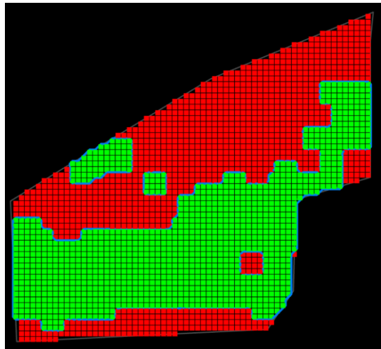
Figure 10 – Example blast with 4x4 minimum size ore block
