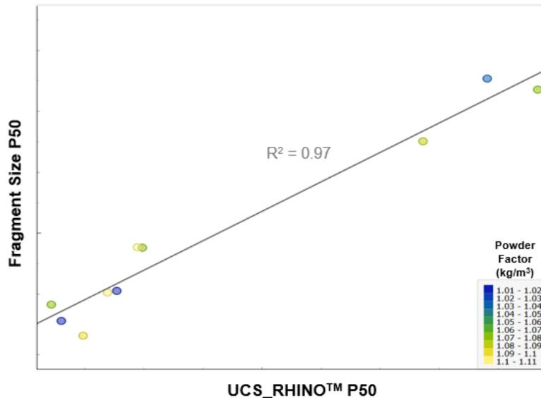
Figure 9. Fragmentation correlation to UCS for a given powder factor. The median fragment size shows a strong linear correlation to the median UCS measured in ten grade blocks that were blasted with similar powder factors.
