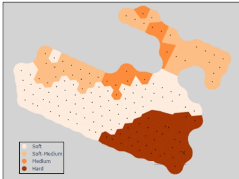
Figure 8. Blasting domains created by clustering blastholes with similar UCS values. In this example four domains have been identified. The number of domains can be adjusted according to the number of different explosive types available.
