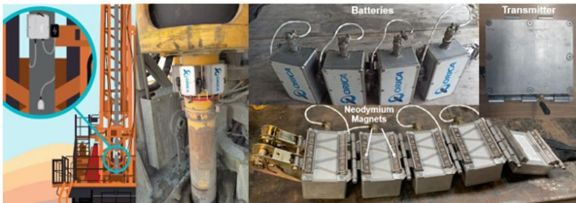
Figure 1. Sensor system deployment. Accelerometers, batteries and radio transmission modules are magnetically mounted at the top of the drillstring.
