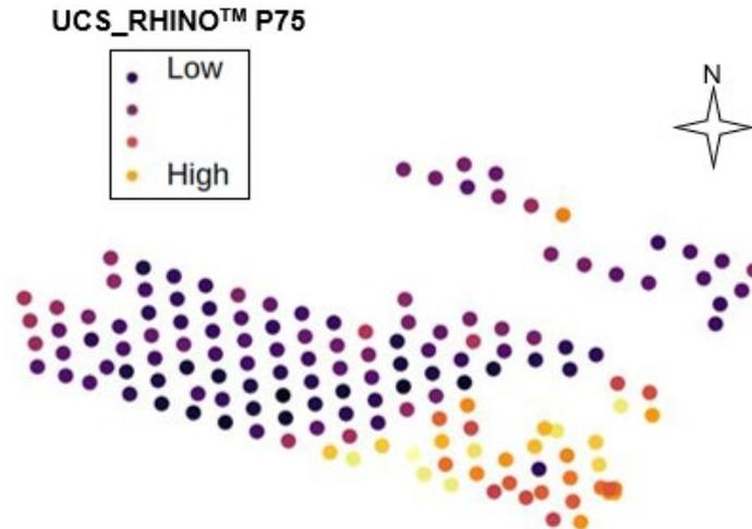
Figure 7. Horizontal variation in rock UCS value. Plotting a colour-coded map of the third quartile UCS value for each blasthole helps visualize the lateral distribution of rock hardness across a drilling pattern. This example corresponds to the pattern shown in 3D in Figure 6. Dark blue indicates low UCS rock, corresponding to the location of the fault. Lighter colours to the south of the fault indicate harder rock.
