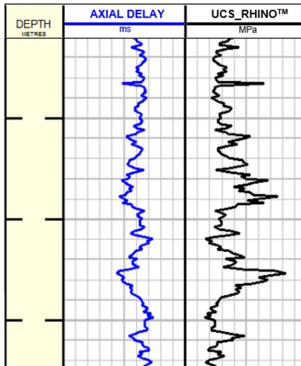
Figure 5. Depth log of measured delay time and rock UCS derived from the delay measurement,
