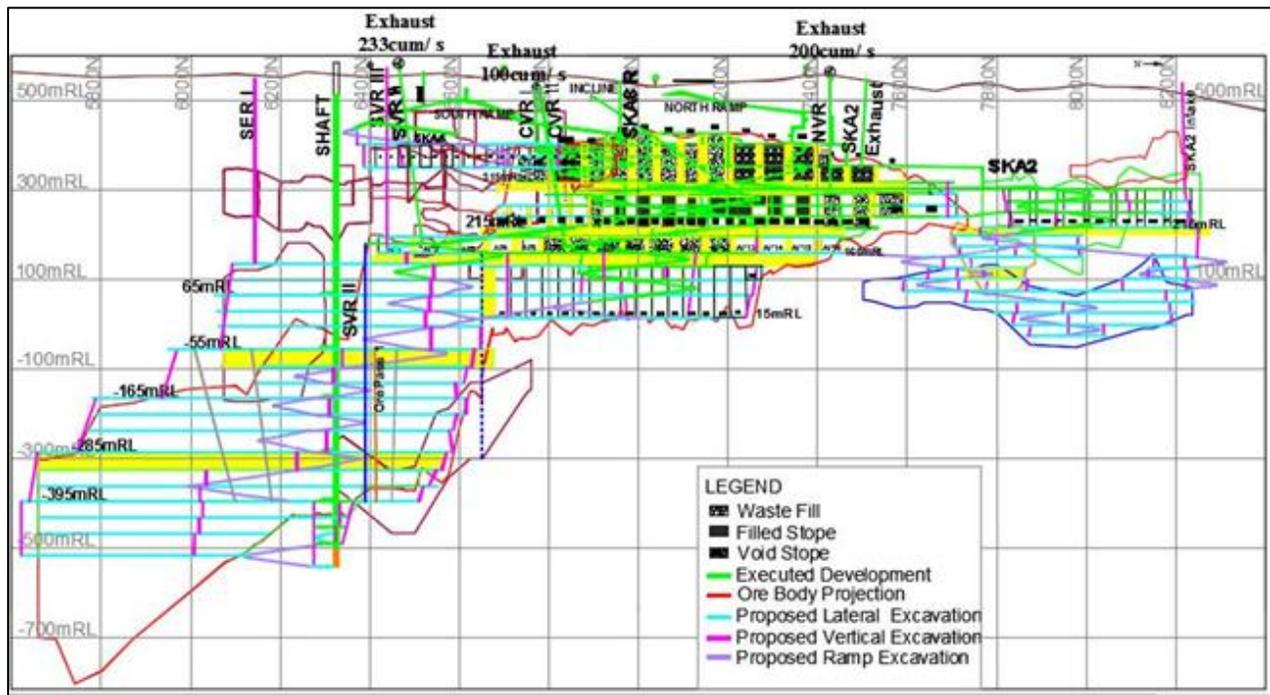
**Figure 1. Longitudinal Section of the mine**
