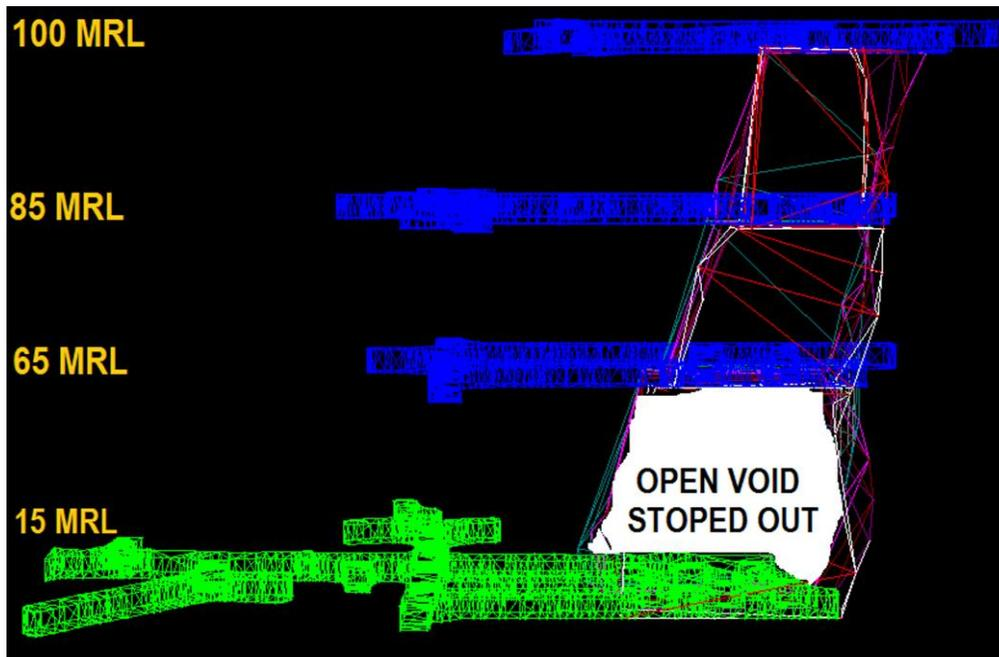
**Figure 2. Current Scenario of the Pillar to be extracted**
