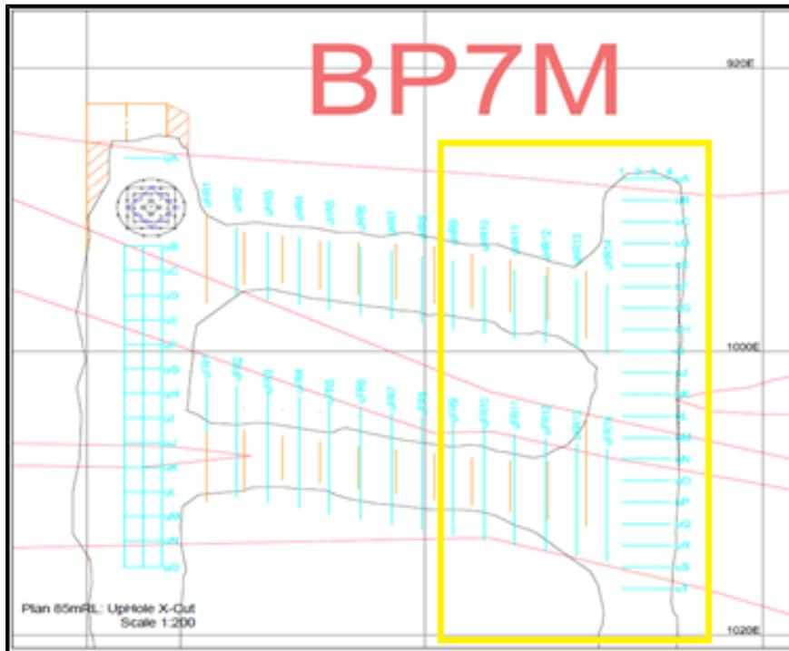
**Figure 6. Demarcation of next blast in Stope**
