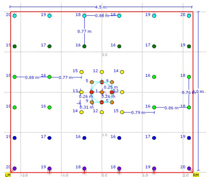
Fig 5: Design using Shotplus™T.
