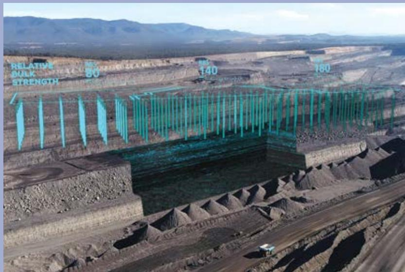
Orica's 4D matches the required energy to rock strength in real time. (Image: Orica)
