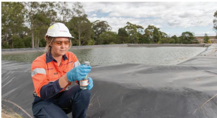
Water quality testing at one of the sealed holding ponds. Water is tested before being discharged to trade waste.
